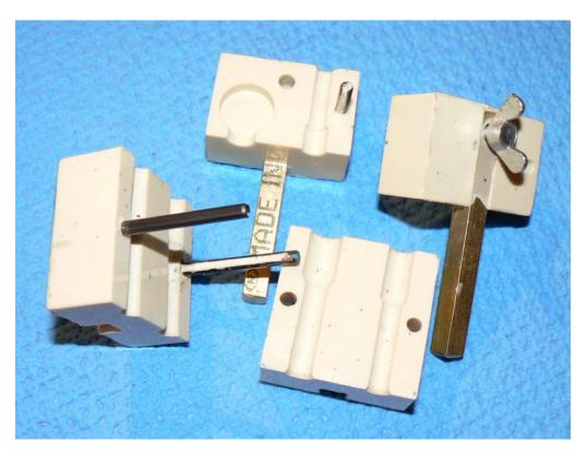
The following illustration shows the insertion tool's two bottom halves. The groove's lower smaller width section clamps the line and the wider upper section provides room for the barb to expand the line. The tool can handle both the 6mm & 5mm lines just by switching sides. The top section will properly align the barb with either of the bottom grooves.
