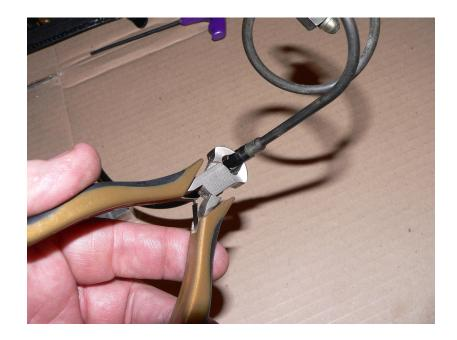
Be very careful to pinch only the line. A nicked barb will leak & must be replaced.
