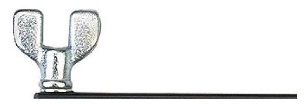
Use the 5/16"(7.94 mm) hole, it should grip fine on either the 8mm plastic or SS braided line. Only tighten the wing nuts enough to hold the line while inserting the barb. Once you get the line gripped by the tool, lay the tool between vise jaws that grip it & let the wing nuts keep the tool from going thru the vise jaws while tapping the barb into the fuel line.
