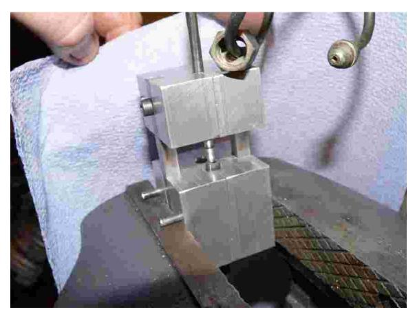
9. Press the top section downward, inserting the barb into the fuel line:
