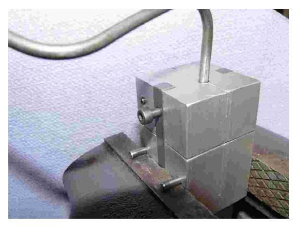
Note that in the above picture the set screw isn't fully tight. The setscrew doesn't need to be tight as the square alignment pins and vice jaws will hold the top closed. The screw is just loose enough for the barbed line or banjo to slip in & out between the halves. This can speed up operation considerably!
