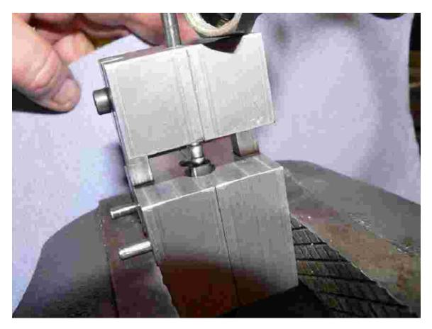
The following picture shows the tool in its closed position, the barb is fully inserted.
