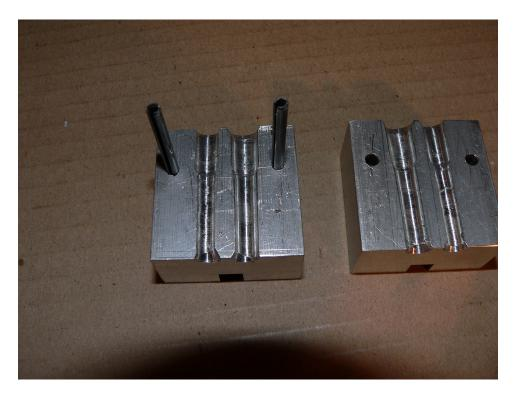
4. Insert the line's end into one side of the bottom section. The line should extend slightly above upper edge. Next slide the other half over the pins and clamp the tool's bottom section in a vice. The round alignment pins will keep the tool from sliding down thru the vice jaws.
