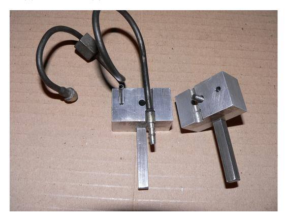
8. Squeeze the two halves of the top section together, clamping the barb or banjo between them. Then slip the alignment pins into the square grooves along the bottom section. The vice jaws holding the bottom half will also hold the top section together by the square alignment pins.
